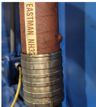
Figure 1: Hydraulic hose protrusion requires replacement
