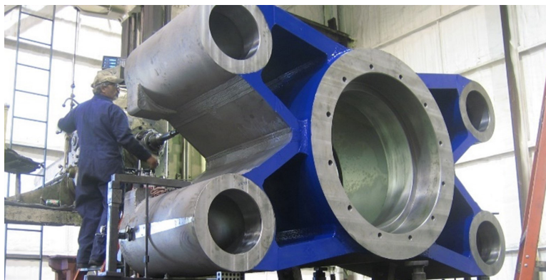
Figure 6: Fabricating a new cross head at Campbell
