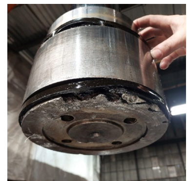
Figure 3: Damaged pull back piston
