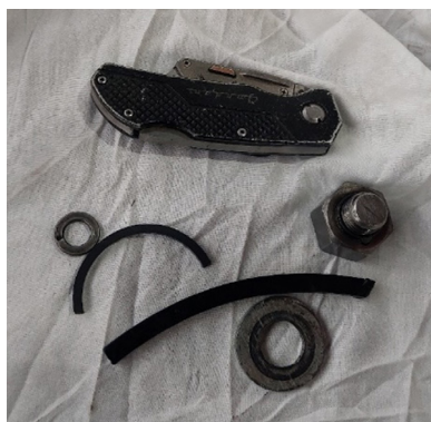
Figure 2: A few of the items found in the bottom of the oil tank
